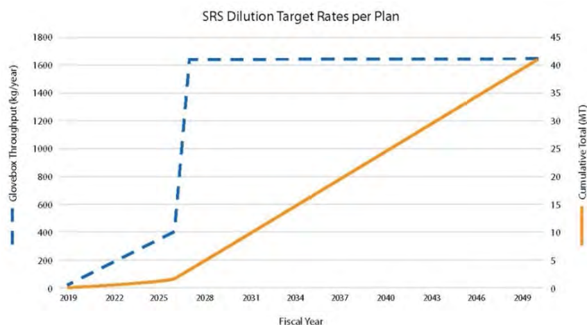
FIGURE 3-7 Graph of the dilution rates and cumulative production of diluted surplus plutonium as a function of time.
